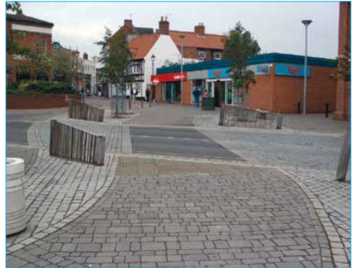
Gainsborough Riverside Walk. In this case the installation of guard rails was deemed to be necessary. However, a distinctive design has been used, using high quality materials to complement the design and materials of the rest of the street furniture along the Riverside Walk. Either side of the crossing, on the carriageway, different materials indicate to drivers to slow down for the crossing. The crossing itself follows the pedestrian desire line, and draws pedestrians into the shopping areas in the centre of Gainsborough. It also has well-maintained trees, which are an appropriate species in terms of size and shape for the area.
