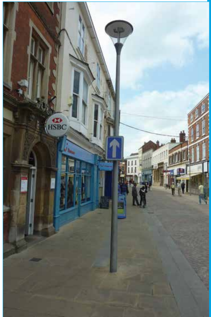
A one-way sign has been mounted on a lighting column in the recently completed Market Place Scheme in Gainsborough.
