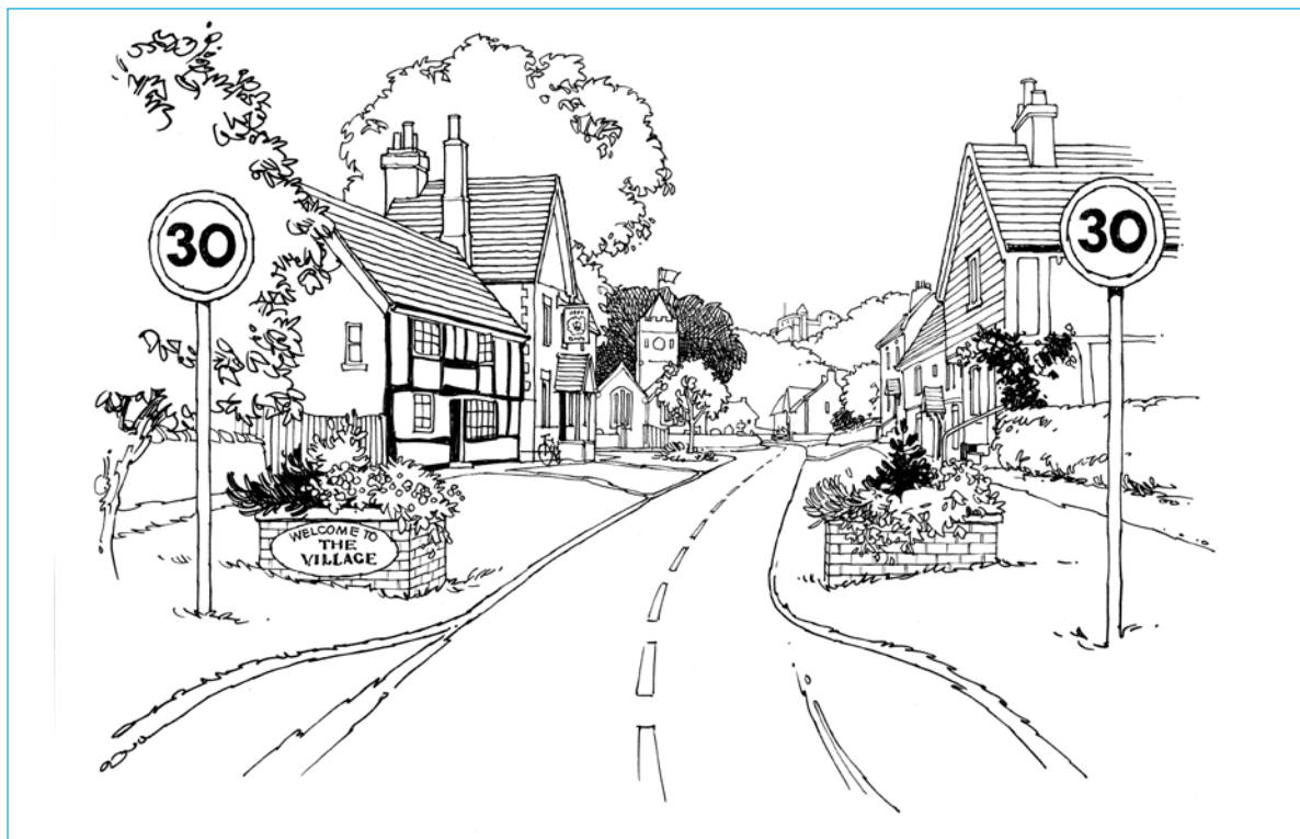
This illustration is an uncluttered village entrance. Note the narrowing of the road as a technique for reducing vehicle speeds without the need for further signage. Illustration by Print Talk.
