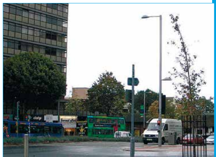
Maid Marian Way, Nottingham. Note the street lighting column, with traffic signals attached, to the right of the image. Note also the lack of pedestrian guard railing.
