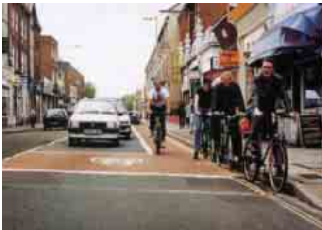
Figure 7/1 – Advanced Stop Line
